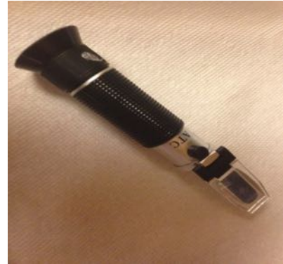
Refractometer / Brix meter used to measure the brix of fruit juice.
